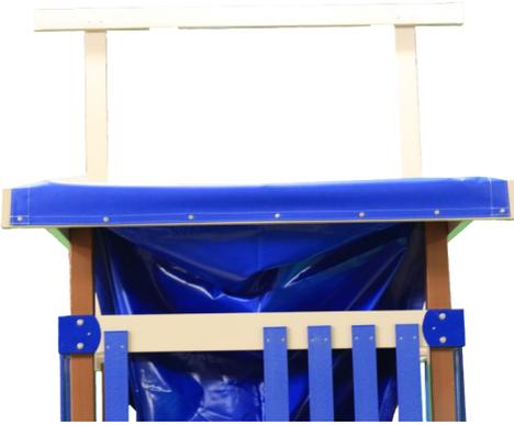
Center the canopy on the #3 2x6 and fasten with 7 - canopy screws
