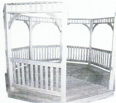
#18 - With posts and railing installed and secure, position door assembly in opening. Center door jamb on post.
