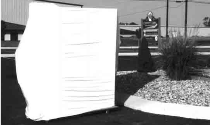
#2 - Materials banded and wrapped on skid.
