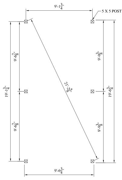
$10' \times 20' \text{ POST LAYOUT PLAN}$ SCALE: 1/4" = 1'-0"
