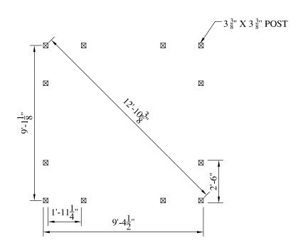
$\frac{10'}{\text{SCALE: }1/4"} = \frac{10'}{1-0"} \frac{\text{WOOD POST LAYOUT PLAN}}{\text{PLAN}}$
