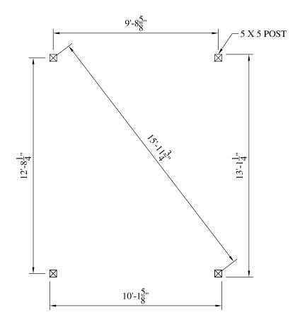
$\frac{14}{\text{SCALE: }1/4}$ " = 1'-0"  $\frac{1}{1}$  POST LAYOUT PLAN
