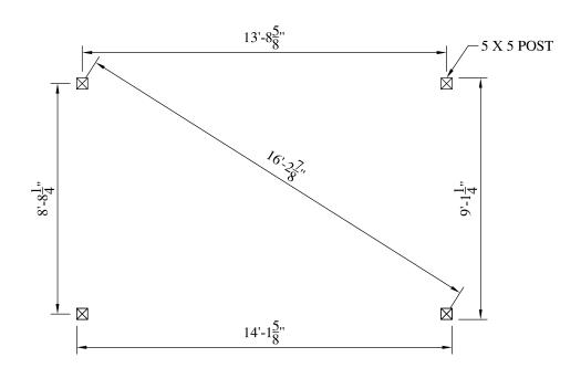
$\frac{10'}{\text{SCALE: }1/4"}$   $\frac{15'}{= 1'-0"}$  POST LAYOUT PLAN
